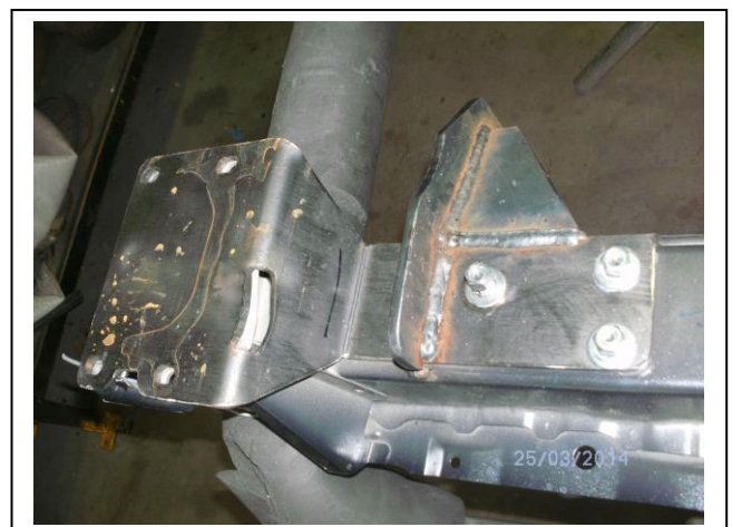
Figure 4: Install ECB mount to rear of bumper support using two M10 x 35 bolts on wire.
