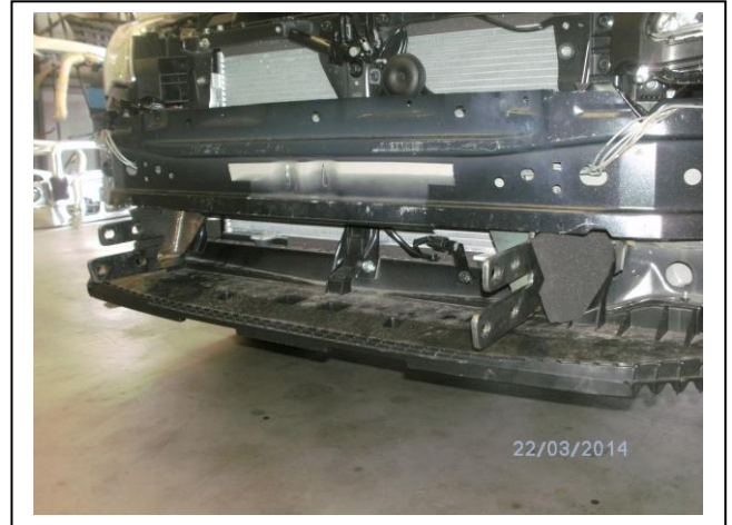
Figure 6: Mounts fitted to vehicle.
